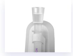
Figure 20: A column reservoir on a qEVoriginal Legacy column.
