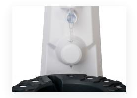
Figure 7: The nozzle tip centred over the flush hole. Note that for the side of the carousel that holds 2 mL tubes, the flush hole will be on the right of the central well channel. For the other side of the carousel that holds 5 mL tubes, the flush hole is on the left of the central well channel.
