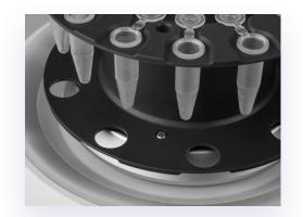
Figure 19: The alignment pin correctly engaged in the carousel.
