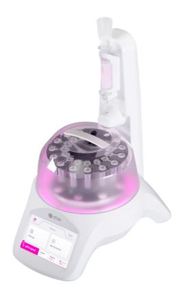
The AFC measures the volume of each fraction by weight as it fills with liquid eluting from the column. When the designated threshold weight is reached, the fluid flow is automatically stopped to prevent dripping of fluid during repositioning of the carousel.
