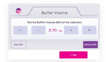
Figure 17: The Buffer Volume menu allows you to set the buffer volume of the collection run. Default BV sets the volume to the recommended buffer volume, while Zero BV sets the buffer volume to zero. Press -/+ to adjust in small increments and --/++ to adjust in large increments. Press Set to save your parameters and return to the home screen.
